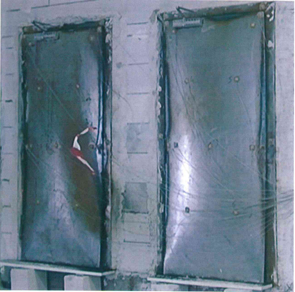
Photo C3: Unexposed side of the test specimens after the test.
